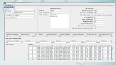
gas pressure is controlled by the valve at the end of each gas flow line. The valves automatically control and maintain either zero differential pressure or a finite definite pressure difference. Absolute pressure remains close to the standard pressure. The inlet and outlet flow rates and humidity are measured. The water vapor transmission rate through the sample is computed using the following relation.
